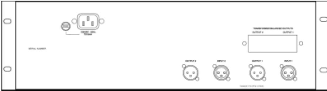
The input and output connectors are wired on female and male XLRs respectively, wired as follows:
